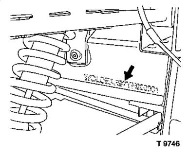
The vehicle identification label is bonded to the body in the front compartment.
